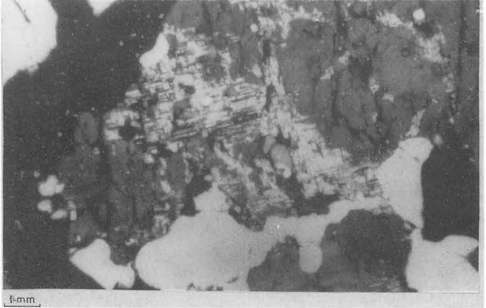
Fig. 8 Photomicrograph showing K-feldspar porphyroblast with perthitic texture.
