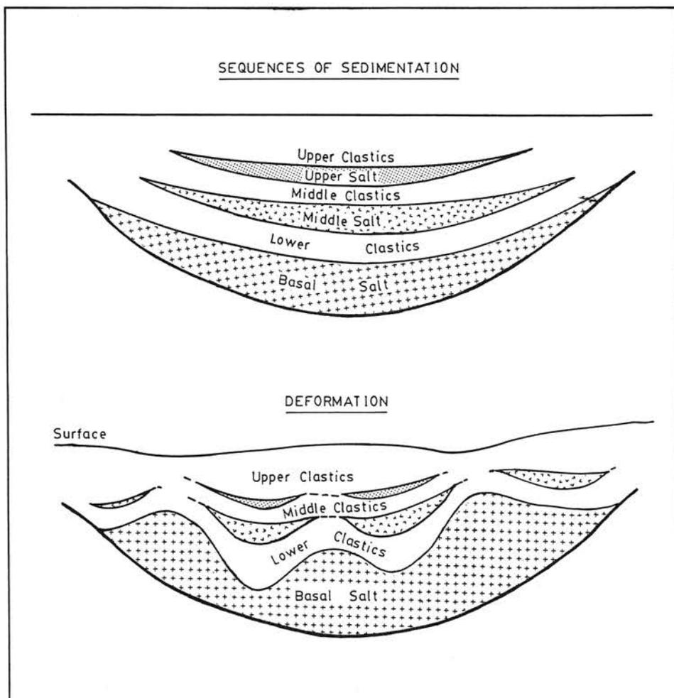
Fig. 9 Sequences of sedimentation and their post-depositional structural deformation (Modified after Hite, 1982).
