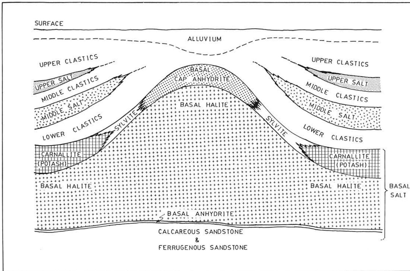
Fig. 12 Proposed model of secondary changes of evaporitic facies (Modified after Hite, 1982)
