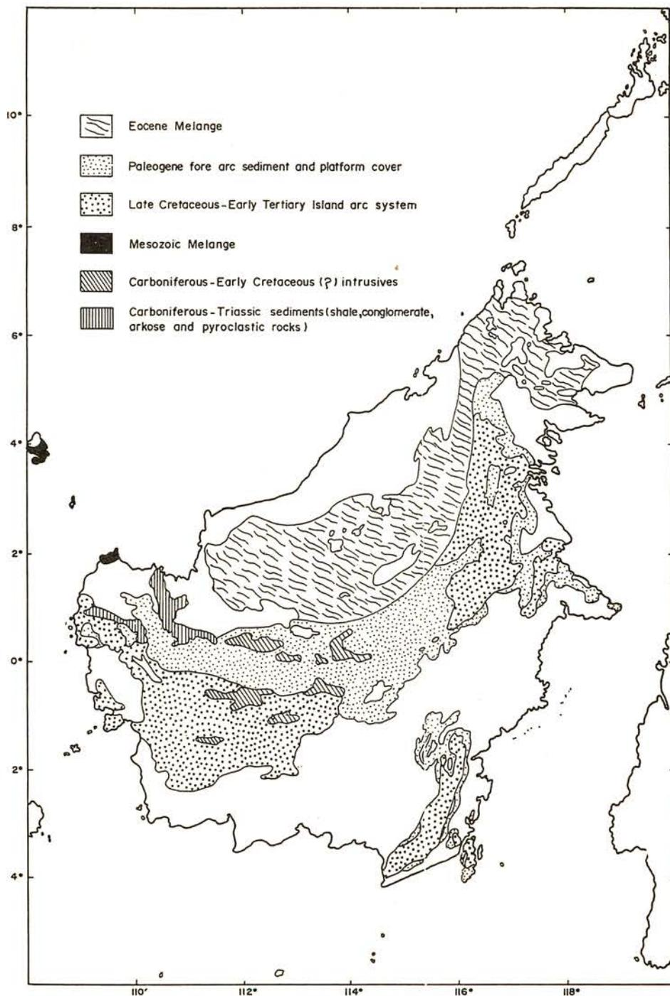
Fig. 2 Proto-Kalimantan terrane map, which includes the Pre-Late Triassic part of Carboniferous-Early Cretaceous intrusives, Carboniferous-Triassic sediments and possibly the melange of Natuna (Hartono and Tjokrosapetro, 1984).
