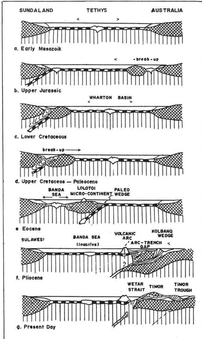
Fig. 27 Evolutionary scheme to explain the geology and structure of Timor (Barber, 1981).
