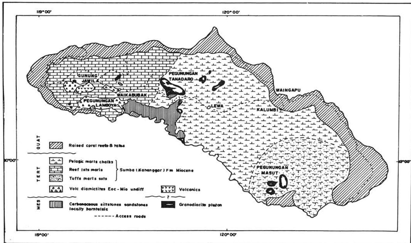
Fig. 11 Generalized geological map of Sumba (von der Borch et al., 1983) to show units belonging to the Sumba terrane.
