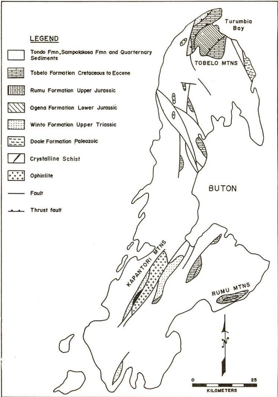
Fig. 7 Buton terrane map, which includes all Pre-Cretaceous geologic units (Hartono and Tjokrosapetro, 1984).
