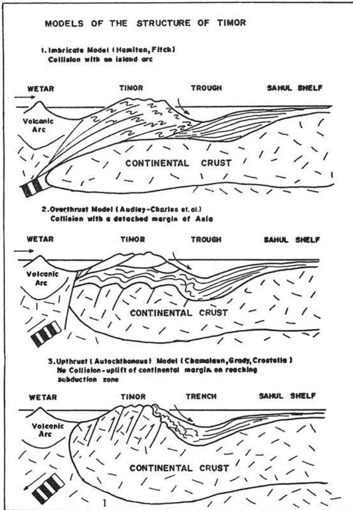
Fig. 26 Models of the structure of Timor (Barber, 1981).
