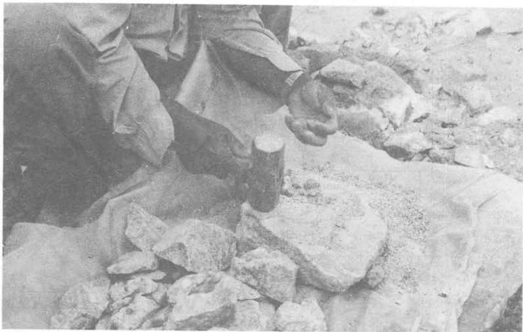
Plate 3: Detached cassiterite-bearing rock is pulverized with a hammer to liberate the cassiterite from the gangue.
