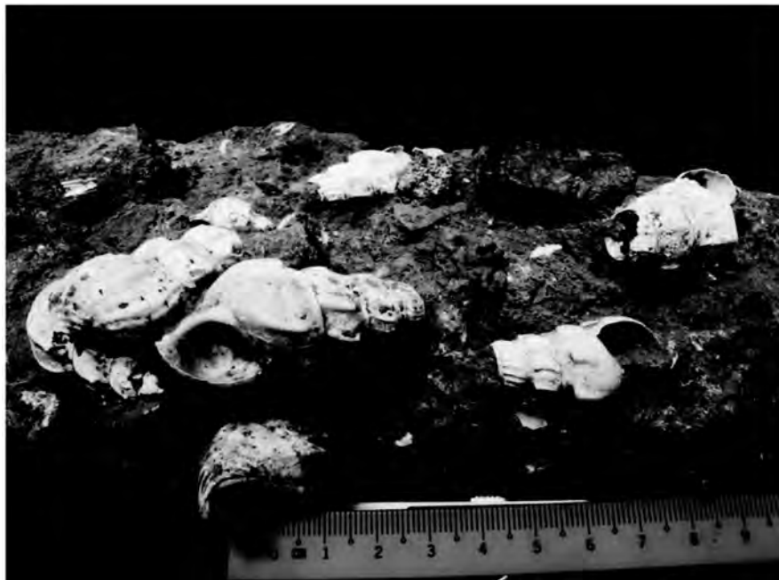
Figure 3. Hand specimens of porous calcareous sediments with weakly aligned shells of Brotia costula , fragments of hematite and baked red clay.
