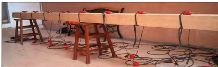
Figure 1: The test array and wave travel for ultraseismic test.
