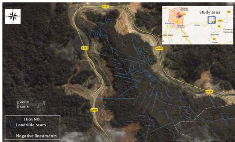
Figure 1: Relict landslide scars and lineaments along the natural slope.
