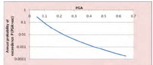
Figure 3: Hazard curve for line source using Boore, Joyner and Fumal attenuation expression.
