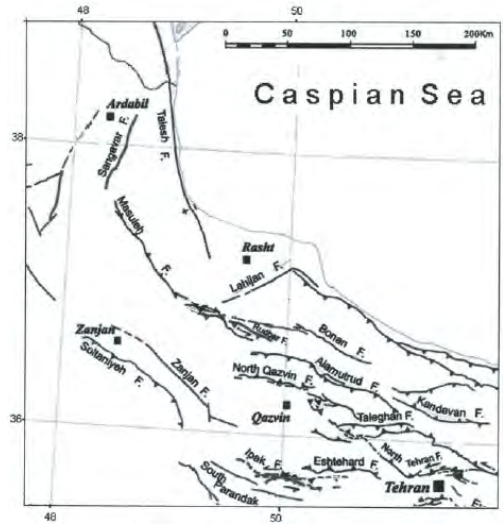
Figure 1: The active faults of Gilan province (IIIES, 2002)
