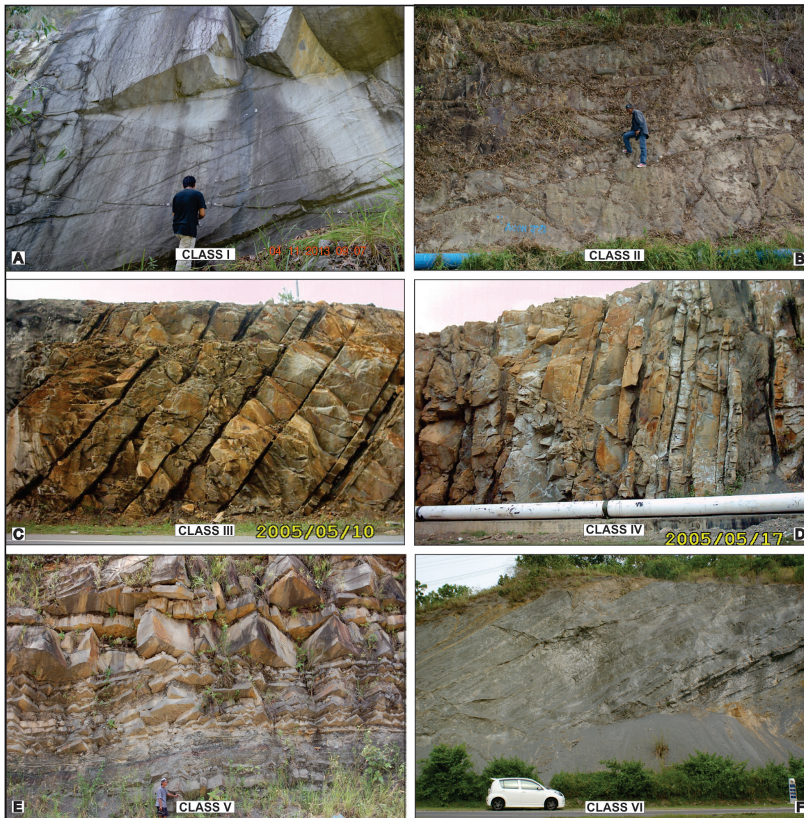
Figure 2: Modified Slope Mass Rating (M-SMR) classes for selected slopes. A – Slope BS; B – Slope LP; C – Slope TS2; D – Slope TS1; E – Slope B; F – Slope TH.
