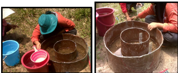
Figure 3: Field infiltration test using double ring infiltrometer.
