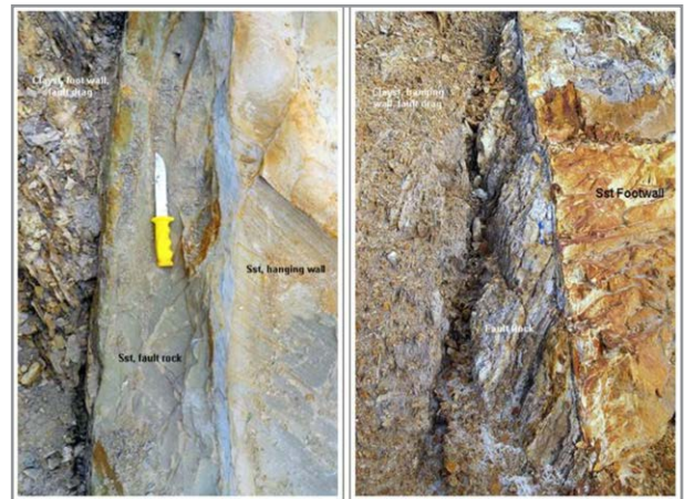
Figure 8: Lateral fault sealing is further complicated by the presence of fault rock common for brittle material. Clay gouging is observed between claystone and fault rock, and between fault rock and the tectonically unaffected part of the sandstone bodies. In the studied outcrop, fault rock is formed in major sandstone bodies, regardless of in hanging wall, or footwall position. From Kessler et al. (2010). The authors intend to further investigate clay gouge sealing capacity, and calibrate the outcrop data with modeling tool such as FaultRisk™.
