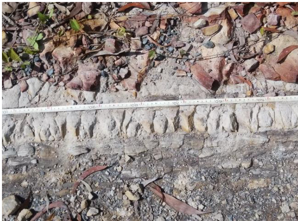
Figure 1: Measuring joint spacing along strata using measuring tape.
