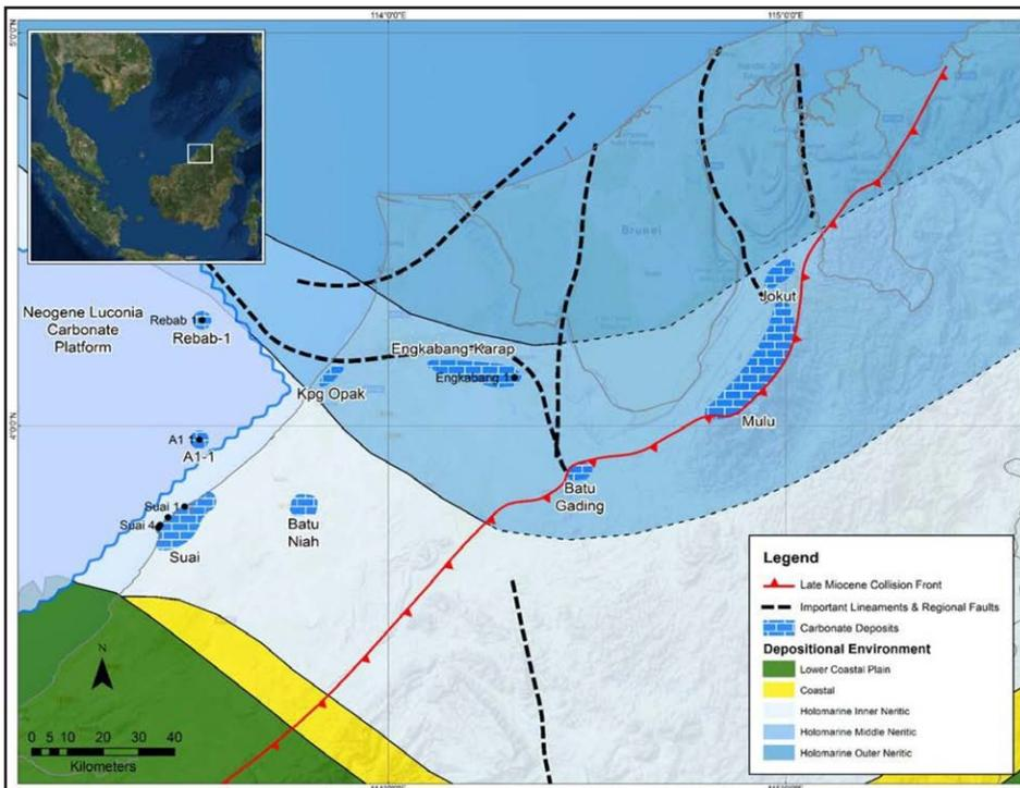
**Figure 21:** Regional palaeo-environment map of northern shore of Borneo with carbonate distribution discussed in this paper illustrating the variation in depositional environments at Cycle I time (Late Oligocene to Early Miocene), which was extended offshore integrating data from Abdullah *et al.* (2015).
