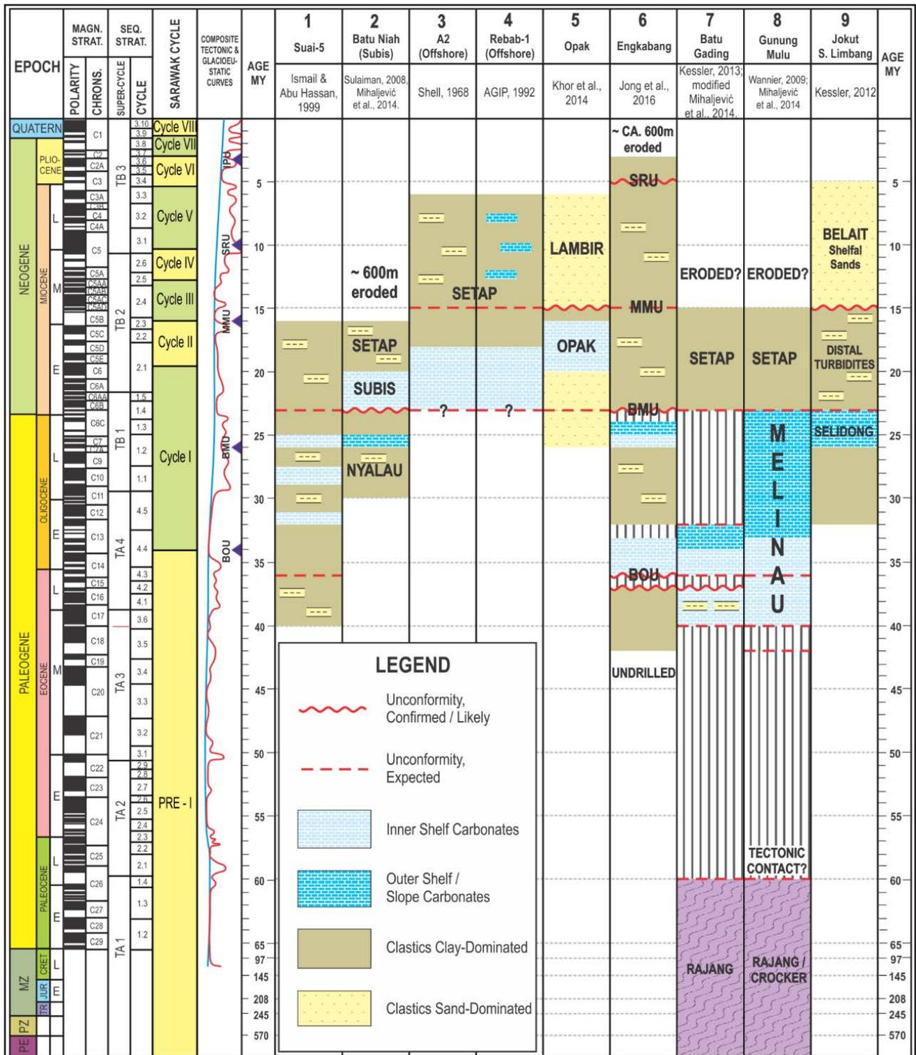
**Figure 17:** Correlation of important carbonate deposits from well and outcrop investigations in NW Sarawak. The correlation suggests the development of an older carbonate system which was separated from the younger one by the BMU. The tectonic and regional significance of Base Oligocene Unconformity (BOU), Base Miocene Unconformity (BMU), Middle Miocene Unconformity (MMU) and Shallow Regional Unconformity (SRU) as annotated has been discussed recently by Kessler & Jong (2016b).
