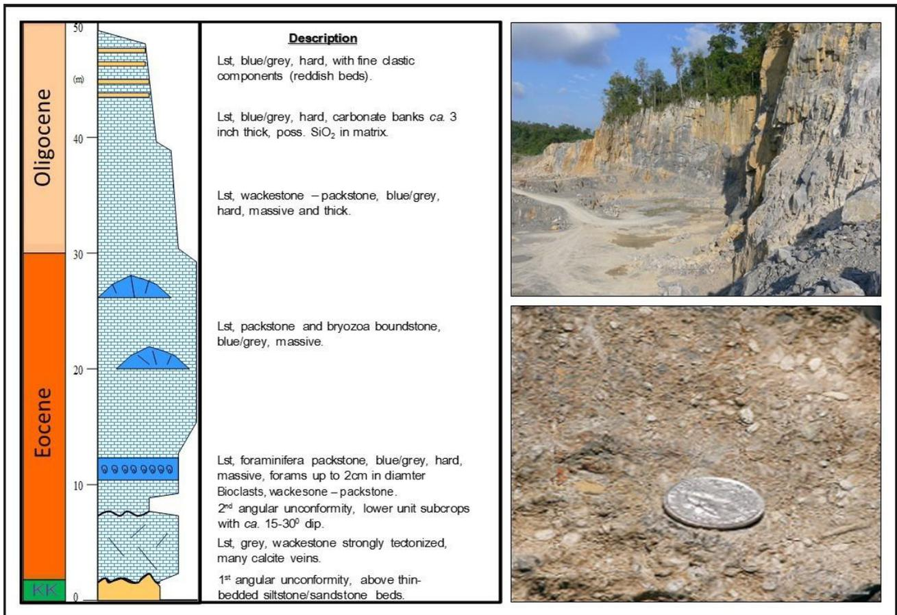
**Figure 11:** Vertical profile of Batu Gading limestones (Hollystone quarry, after Kessler, 2013). Top right: The Hollystone quarry is located in the vicinity of the discussed Baram-Luconia/Tinjar tectonic segments, imbricated between older Kelalan metamorphics. However, there is no indication that the Batu Gading limestone has undergone metamorphism. Bottom right: Foraminiferal packstones in Batu Gading limestones of a ramp facies. These carbonates appear to contain always some clay component.
