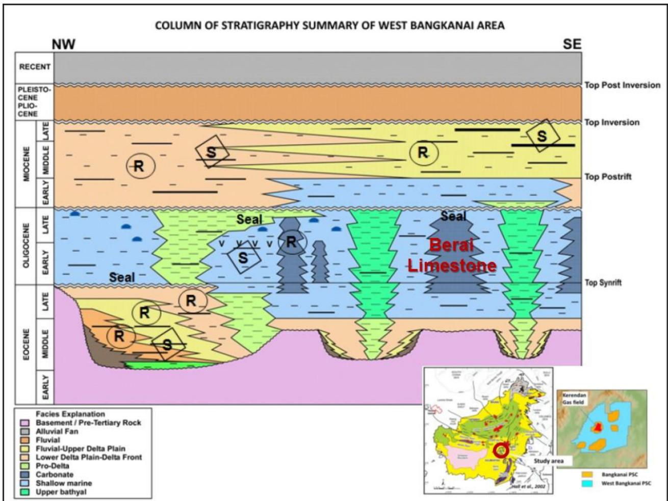
**Figure 15:** Stratigraphic column of Bangkanai and West Bangkanai area, onshore Upper Kutei Basin (after Subekti *et al.*, 2015).
