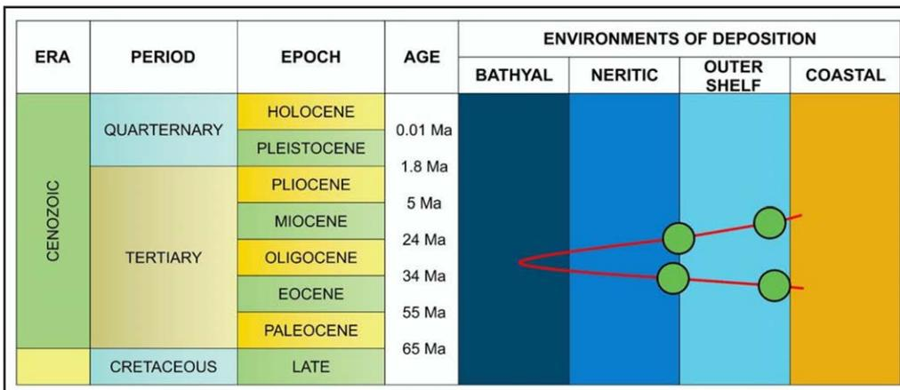
**Figure 25:** Estimate of sea-level change (red line) from Late Eocene to Mid Miocene inferred from water depth indications of studied carbonate deposits. Green circles show the occurrence of carbonates as the foredeep area drowned, and later re-emerged.
