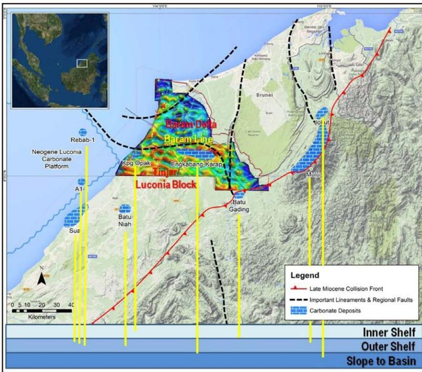
**Figure 19:** Distributions of studied carbonate deposits in NW Sarawak with inferred water depths of Late Eocene to Early Miocene carbonate sections at various well and outcrop locations. However, water depth uncertainties remain tentative and deserve further studies. Modified after Kessler & Jong (2016a).
