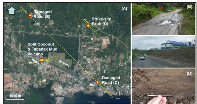
Figure 12: (A) Active strike-slip fault associated with two persistent road depressions aligned NW-SE at Lahad Datu town. (B & C) The damaged road sits on Miocene Tabanak Formation. (D) NW-SE trending slickensides associated with sinistral strike-slip fault on the Tabanak Formation. See Figure 10 for location.
