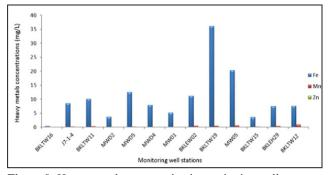
Figure 9: Heavy metal concentration in monitoring wells.
