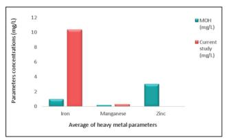
Figure 12: Comparison of groundwater quality for heavy metal with recommended levels by the Ministry of Health for raw water.
