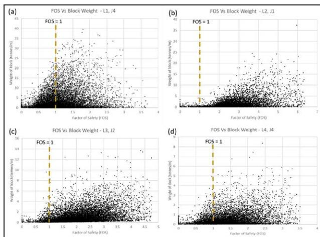
**Figure 8:** Scatter plot for the Factor of Safety (FOS) versus estimated block size. The failed blocks are plotted as points to the left of FOS = 1 line.
