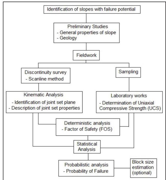
**Figure 2:** Work flow to obtain the probability of failure in this study.
