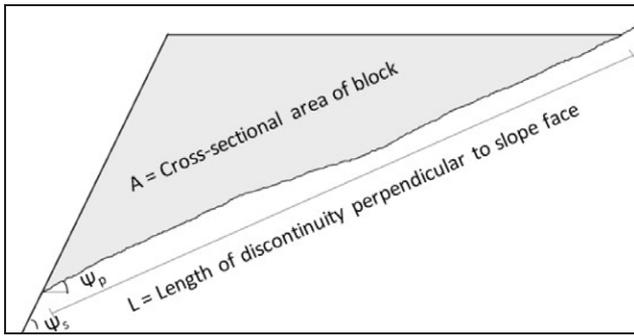
Figure 5: Parameters for calculation in Equation 3.
