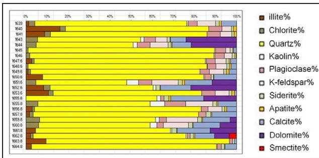
**Figure 10:** Mineralogical compositions of core plugs in a Tenggol Arch field (analysis by AnaMin). Note the relatively high Apatite percentages at 1640 m, 1641 m, 1649.6 m and 1653.6 m.
