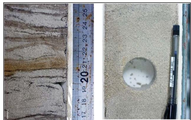
**Figure 9:** Raw core picture from a fresh Tembakau-2 core showing heterolithic (left) and relatively clean massive facies (right).
