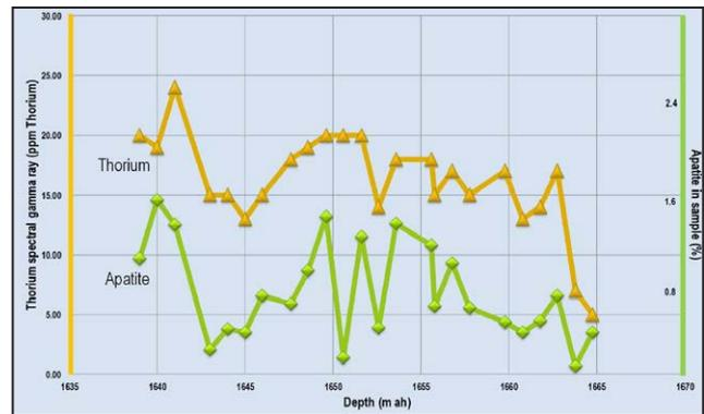
**Figure 12:** Correlation between apatite content (green curve, in sample percentage), and Thorium on spectral gamma ray log (golden curve, converted to ppm Thorium) from a Tenggol Arch field, both plotted against depth in meters along hole. Apatite (present as isolated heavy mineral grains, as well as in rock fragments) is inferred to be the host of observed anomalous radioactivity.
