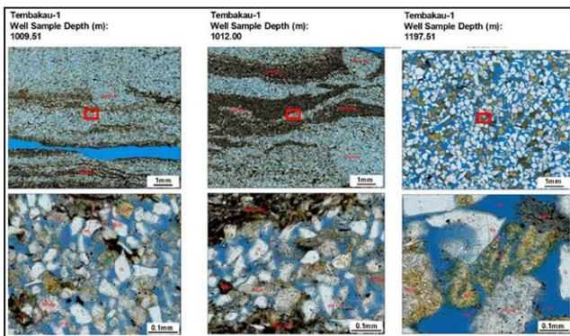
**Figure 6:** Heterolithic clastic hot sand samples as shown above from I-10 interval, Tembakau-1, are very well-sorted, and mostly fine sands. Surprisingly, most grains are sub-angular suggesting deposition relatively close to the provenance. Likely the sediment did not form solely in an aqueous environment. Wind transport may also have played a role. The highlighted areas in the upper photos are the location of the magnified pictures immediately below.
