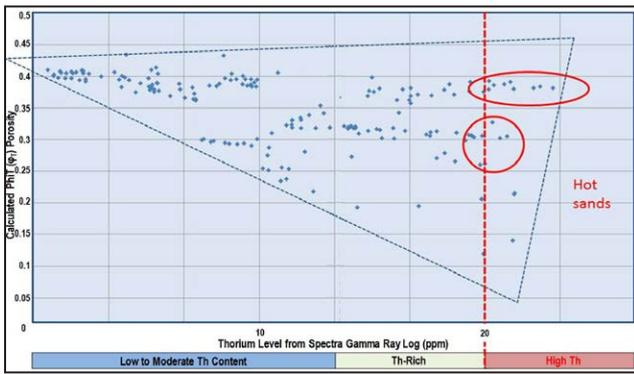
**Figure 13:** Calculated porosity and Thorium radioactivity. The dashed red line corresponds to 20 ppm Th, and gamma radiation levels are shown on the x-axis. The hot sands in the right corner are found within the I-10 sequence of Tembakau-1 exploration well, and in different porosity classes.
