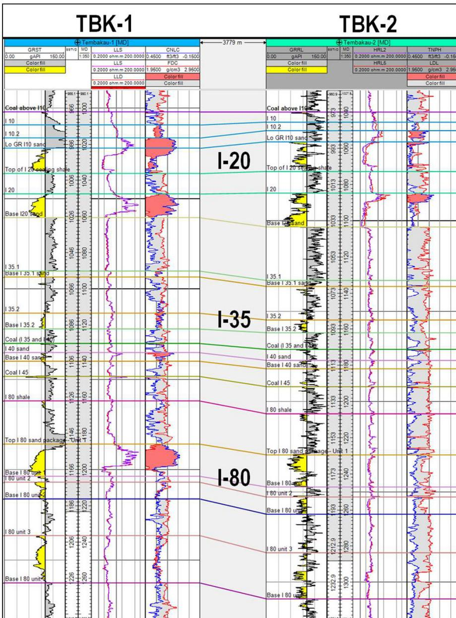
**Figure 14:** Correlation between neighbouring wells (Tembakau-1, Tembakau-2) using Thorium gamma ray responses. It could help refine reservoir modeling and sub-seismic wireline log correlation.
