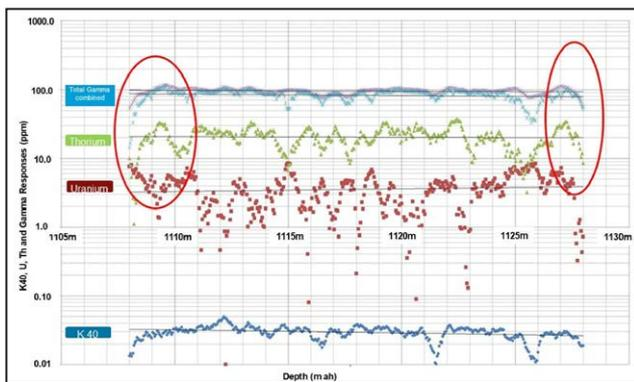
**Figure 11:** Hot sands, I sequence in Tembakau 2. Total gamma (upper greenish blue) is influenced by Thorium (green), causing peaks that are not related to K40 (lower blue curve as shown). Uranium content (red-brown) being low, has no influence on the composite signal.
