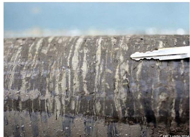
**Figure 8:** Raw core picture from Tembakau-2, Core 1. The thin, 1-5 mm (with a key for scale) grey gas-bearing sand intervals are flasers, and are intercalated between soft clay beds. The sands however, are very clean and do not contain any significant amount of clay.
