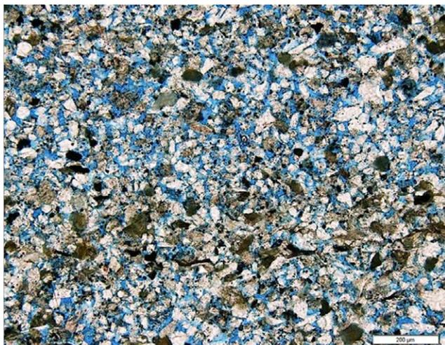
**Figure 7:** Thin section from a Tenggol Arch field core at depth 1634.37 m (K sequence). Typical heterolithic facies formed by sub-angular, yet in general well-sorted quartz and dark and greenish components, likely minerals of the apatite family as well as chlorite and possibly glauconite.
