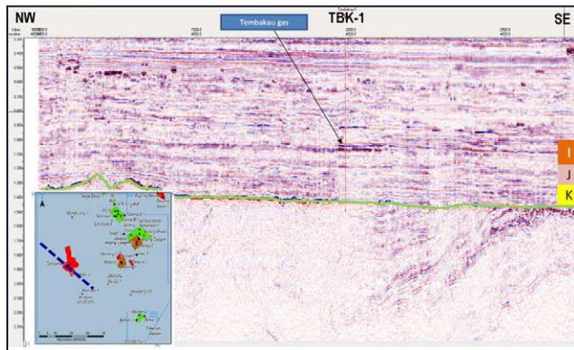
**Figure 3:** A seismic section of *ca.* 50 km length running NW-SE on the Tenggol Arch with approximate line location shown on the inset map. The geology can be divided into (bottom) a strongly deformed basement section, with an isopachous Neogene drape above. The Basement unconformity is highlighted in green. A marked amplitude anomaly in the centre of the picture indicates the presence of gas. The stratigraphic group intervals, I, J, K are annotated.
