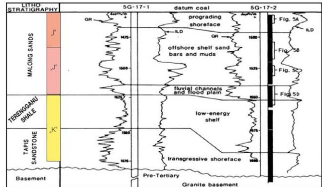
**Figure 4:** Log correlation of 2 Malong wells and facies. Several high gamma ray peaks might represent hot sands, but this remains speculative in absence of spectral gamma ray logging (from Madon, 1990 and modified after Ibrahim & Madon, 1990).
