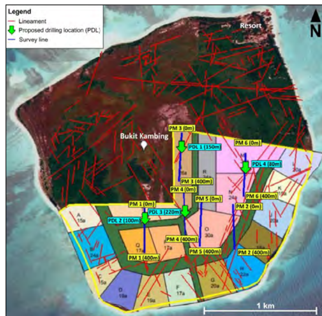
Figure 5: Four proposed drilling locations (PDL) were suggested at Mengalum Island, Sabah plotted on Google Earth image overlay with land lots for future development.
