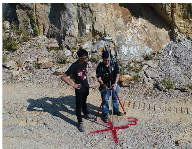
Figure 3: GCP marked in red and GPS equipment set up.
