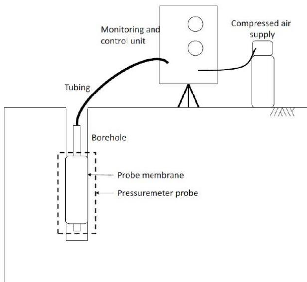
Figure 1: Instrument of pressuremeter test.
