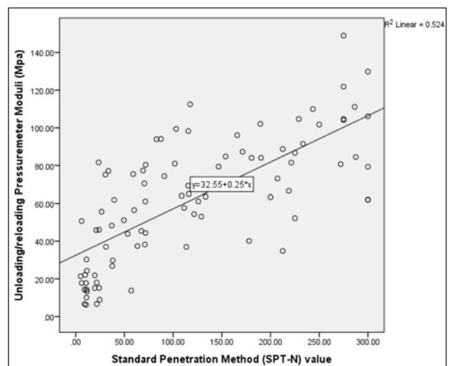
**Figure 5:** Unloading/reloading Pressuremeter Moduli versus Standard Penetration Method.
