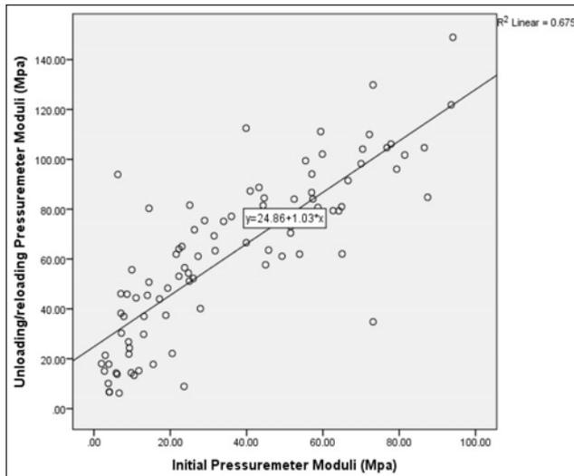
**Figure 6:** Unloading/reloading Pressuremeter Moduli versus Initial Pressuremeter Moduli.
