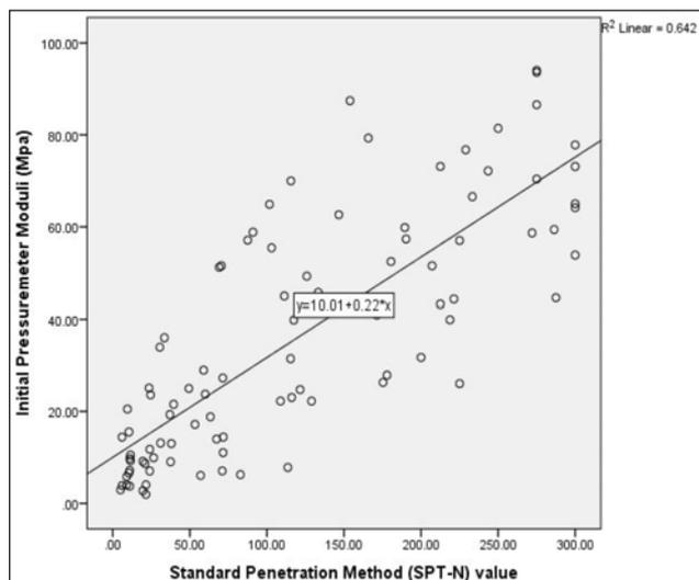
**Figure 4:** Initial Pressuremeter Moduli versus Standard Penetration Method.
