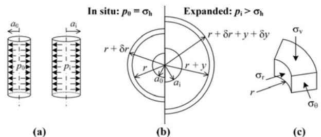
Figure 2: Definitions used in cavity expansion analysis: (a) expansion of cylindrical cavity; (b) expansion of an element at radius  $r$ ; and (c) stress action on an element at radius  $r$  (Likitlersuang *et al.*, 2013).
