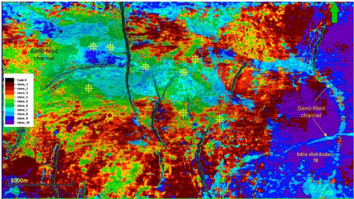
**Figure 9:** Trace-based Waveform classification map, generated by using 10 classes. The map showing an upper delta plain dominated by distributary channels. The channel-fill (class 8 = light blue) is interpreted as sand. This is indicated by well calibration.
