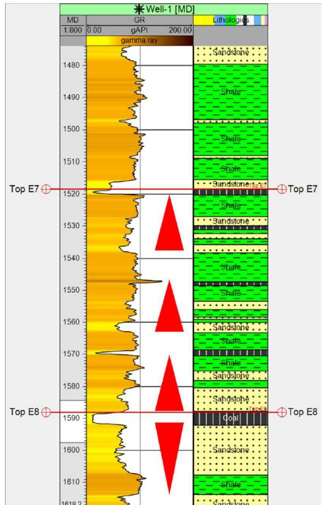
**Figure 6:** Well log display of the upper Group E interval showing sand, shale, and coal intercalation.
