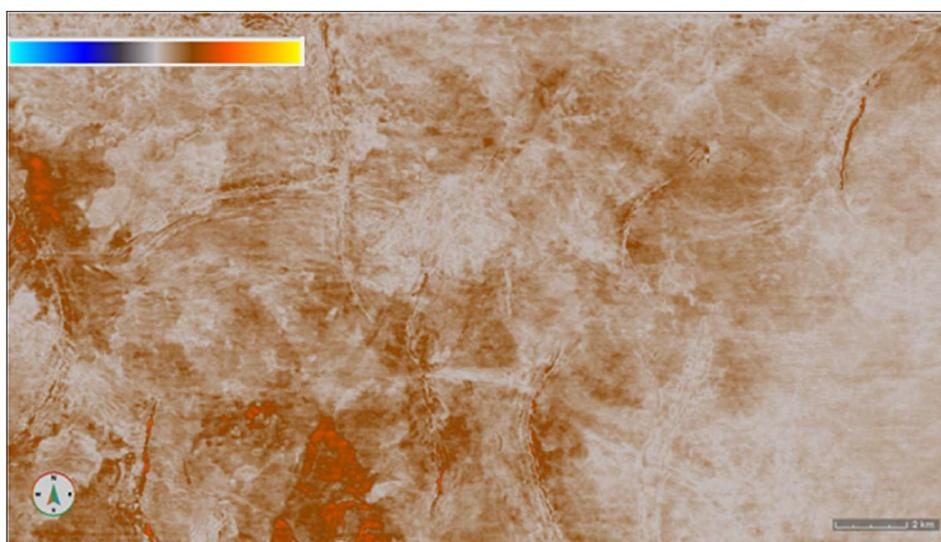
**Figure 7:** RMS amplitude map along E7 horizon. The strong reflection of coal dominates the seismic response and conceals the true geology.
