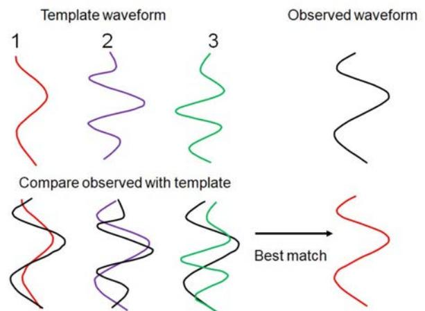
Figure 3: Waveform classification process matches observed trace shapes with a set of model traces and assigns each observed waveform to the most similar trace model (Barnes, 2016).
