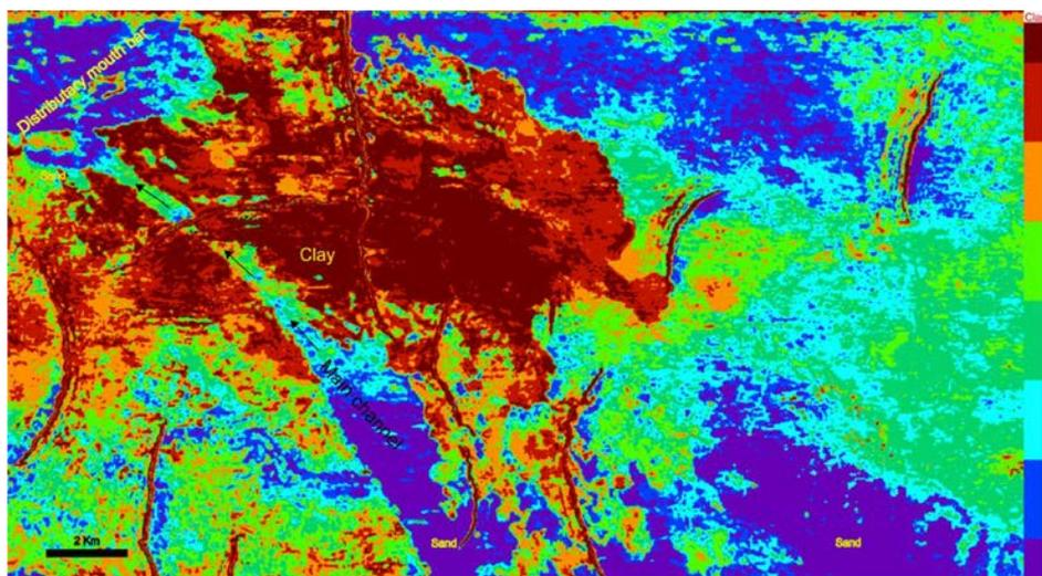
**Figure 8:** Trace-based Waveform classification map, generated by using 8 classes. The map showing the main channel and a distributary mouth bar in the NW corner.
