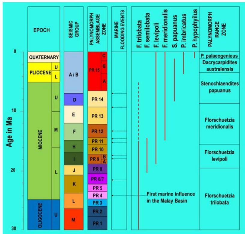
Figure 2: Stratigraphic column of the Malay Basin (Madon *et al.*, 1999).
