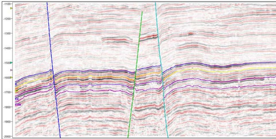
**Figure 5:** Interpreted horizons in the upper part of Group E. These horizons were used as guiding horizons for the waveform classification.
