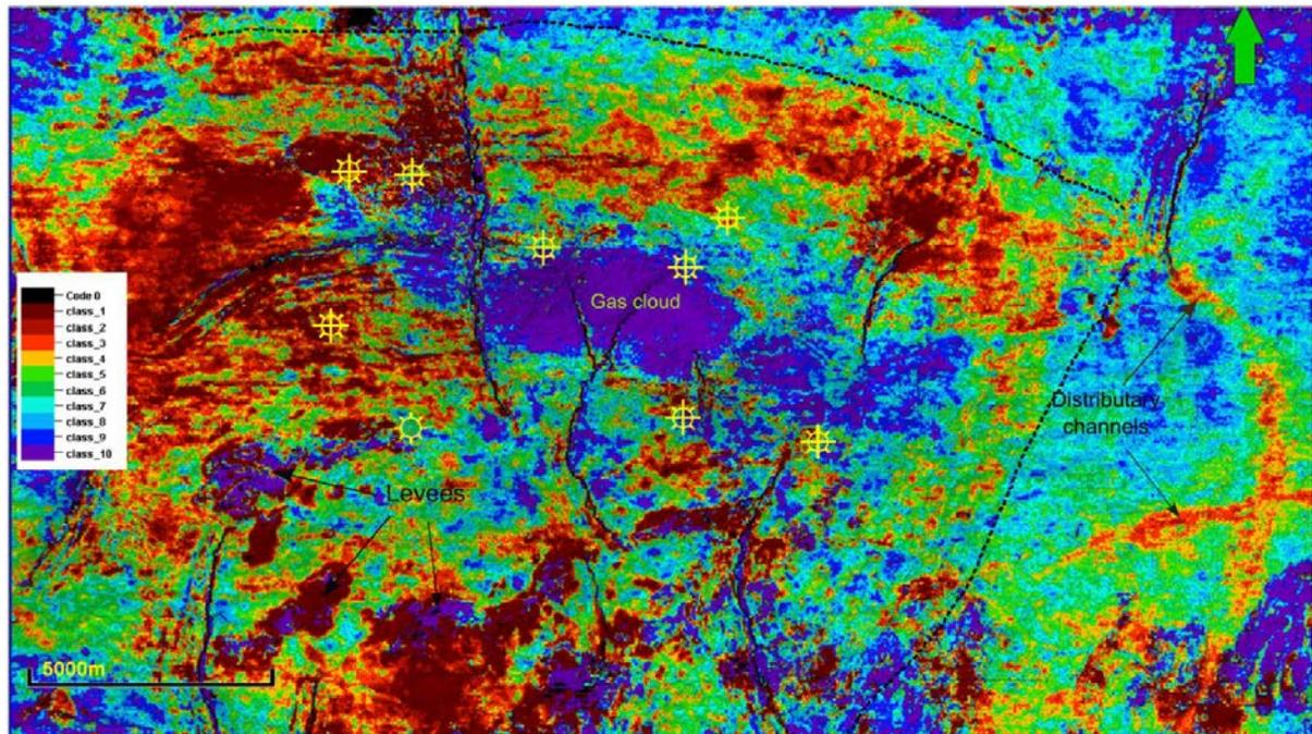
**Figure 10:** Trace-based Waveform classification map, generated by using 8 classes. The map showing a fan-like distributary mouth bar with elongated features interpreted as sub-aqueous levees.
