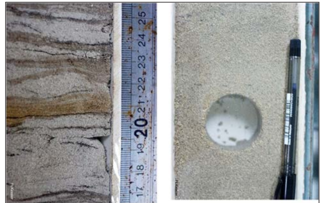
Figure 6: Raw core picture of Group I-10 sand in TBK-2 showing heterolithic facies Type B (left) and relatively clean massive facies Type A (right) (from Jong et al. , 2019).
