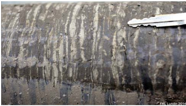
Figure 8: Raw core picture from TBK-2 showing facies Type D reservoir in the top section of Group I-10 sand. The thin (1-5 mm, key for scale) grey and gas-bearing sand intervals are flasers, and are intercalated between soft clay beds. The sands however, are very clean and do not contain any significant amount of clay (from Jong et al. , 2019).
