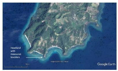
**Figure 5:** Google Earth image of the coast near Sedem (see Figure 3). The arrow is indicating the headland with boulders that have been measured for this study. The image was taken on 28<sup>th</sup> January 2016 and is the view from an eye altitude of 3.39 km; the location of the centre of the image is 6°46'36.51"N, 123°58'49.28"E.
