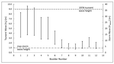
**Figure 7:** Plot of calculated wave heights ranges from Table 2 for tsunami ( $H_i$ ) and storm ( $H_{storm}$ ) waves for each of the boulders (1-12) measured in this study near Namat (boulders 1-6) and Sedem (boulders 7-12). The maximum storm and tsunami wave heights known to have been experienced along this coast are shown for comparison, plotted on the respective axis.
