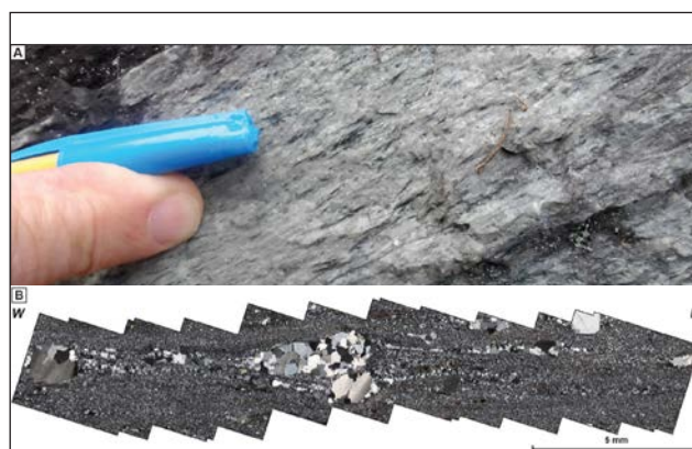
Figure 6: Intensely foliated and lineated, hard siliceous ultramylonitic rocks, Jalan Ukay Perdana 4 (Locn. 2, Figure 2), [420155 354436]; at outcrop (Figure 6a) and in thin section (XPL, Figure 6b). The sense of shear is top-to-the ENE (082°N). The foliation dips 36° to 262°N, the transport lineation is aligned perfectly down-dip. Image BGS © UKRI 2020
