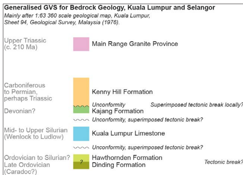
Figure 3: Simplified GVS for Kuala Lumpur and the Selangor region, based on JMG (2011) and the authors' own observations.
