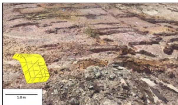
Figure 25: Fracture pattern in relief on ground excavated less than 5 years prior to the photo.
