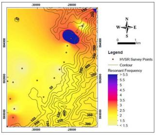
**Figure 7:** Resonant frequency  $(f_0)$  distribution based on 20 points recorded in Balik Pulau.
