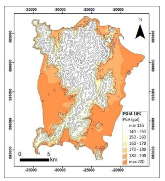
**Figure 4:** PSHA Map of Penang Island showing the probability of events at 10% PE in 50 years (Azmi *et al.*, 2013).
