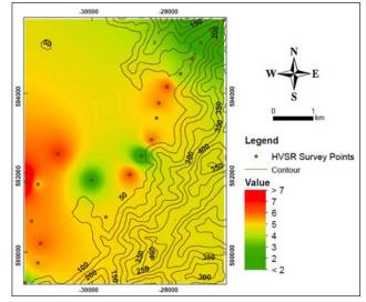
**Figure 8:** Amplification factor  $(A_m)$  distribution based on 20 points recorded in Balik Pulau.
