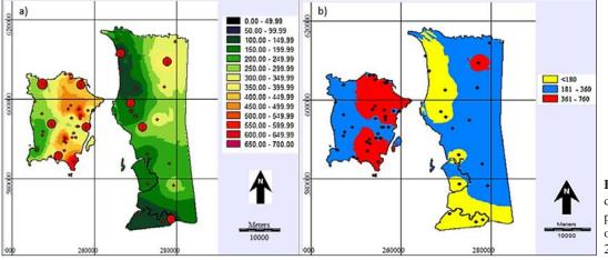
**Figure 2:** a) Vs<sub>30</sub> distribution map b) Soil profile classes based on NEHRP (Tan *et al.*, 2014).
