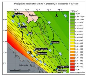
Figure 5: PGA Map of Peninsular Malaysia at rock site condition affected by the Sumatran sources at 10% in 50 years probability of exceedance (Loi *et al.*, 2018).
