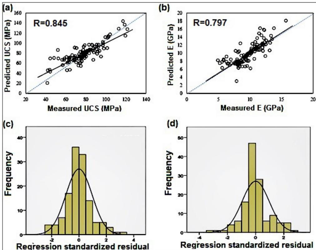
**Figure 3:** The R between measured and predicted values of a) UCS and b) E using the MLR method (models 10 and 20, Table 5); c) and d) the difference between measured and predicted UCS and E from the MLR method, respectively.
