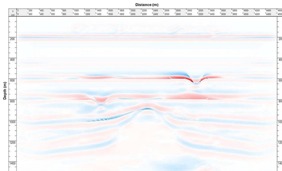
Figure 7: Pre-stack Kirchhoff migrated seismic image in depth domain of ray tracing procedure.
