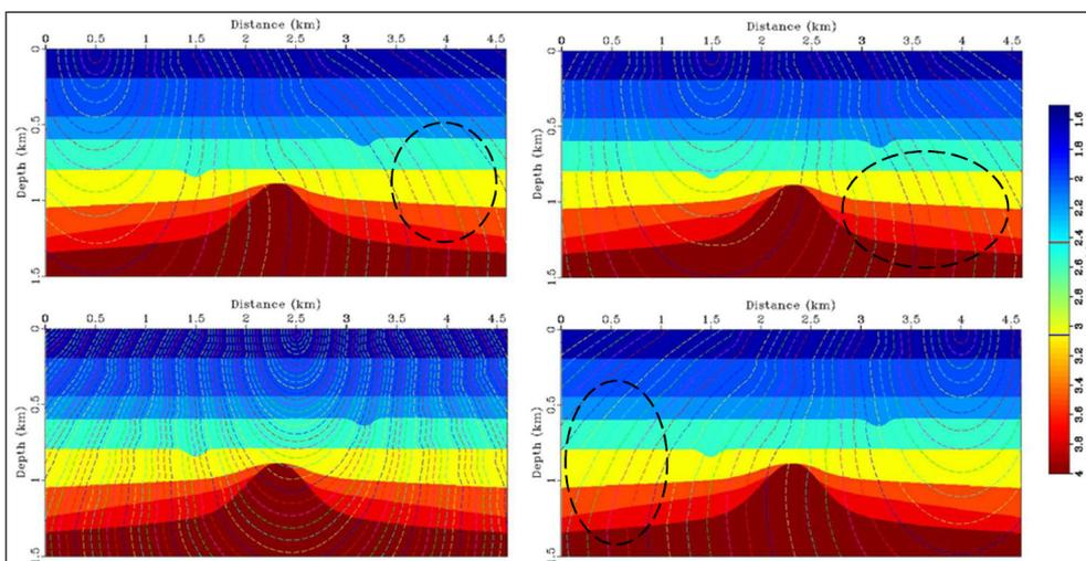
**Figure 4:** Traveltime calculation using fast marching method. The shadow zones have been covered by the wavefronts.
