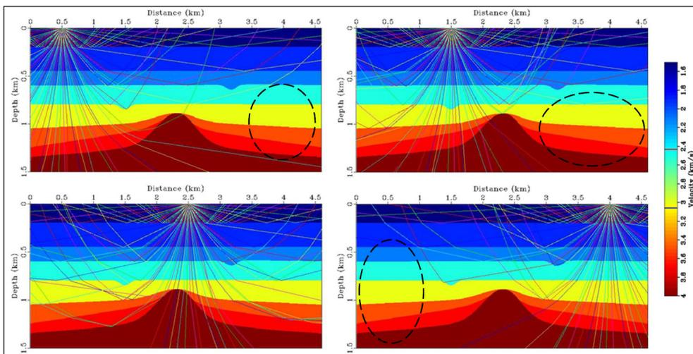
**Figure 3:** Traveltime calculation using ray tracing. The black dotted circles are the shadow zones (area uncovered by the ray path).
