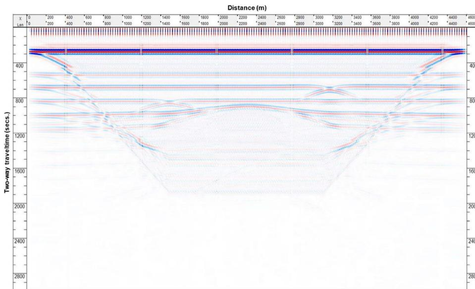
Figure 6: Stacked seismic image from finite different procedure after NMO correction.
