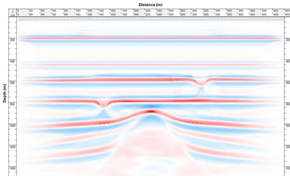
Figure 8: Pre-stack Kirchhoff migrated seismic image in depth domain of finite different procedure.
