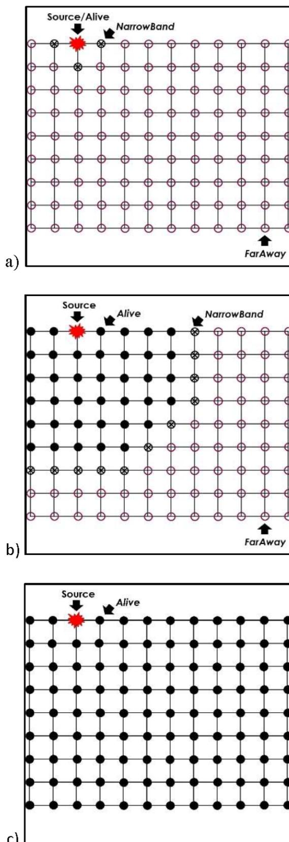
Figure 1: Illustration of complete process of updating traveltime values of every grid point of fast marching method.
