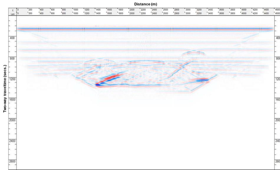
Figure 5: Stacked seismic image from ray tracing procedure after NMO correction.
