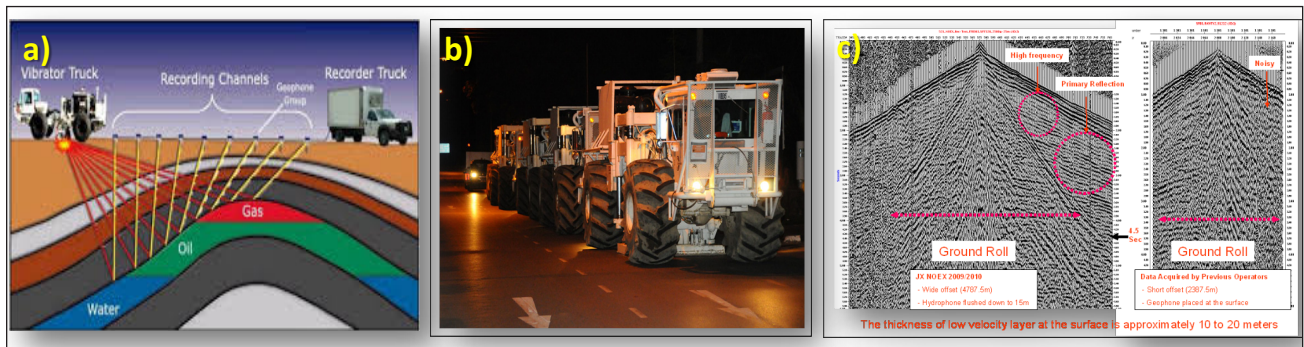
Figure 3: Seismic acquisition operations. a) The objective of seismic acquisition (2D or 3D), is to collect geophysical data on the subsurface hydrocarbon reservoirs within the study area to allow the subsurface targets to be characterised as potential further exploration prospects and for development of the discoveries. Sound wave signals generated by the seismic source travel through the various sub surface rock layers and at points where the rock type changes, reflect back to the surface (red and yellow lines). b) Onshore seismic operations rely on the use of an energy source (impulsive - explosive or non-impulsive) and receivers. The receivers are typically geophones (cables or nodes) which are placed at the surface to record the reflected energy following operation of the energy source. Non-impulsive energy sources include the use of vibrators or vibroseis trucks. Typically, a vibroseis survey involves the use of trucks with vibrating plates that stop at regular intervals along pre-determined survey lines. The truck vibrator plates are compressed against the ground using hydraulic power and vibrated to send energy waves into the sub surface. c) The gathered data is then processed for imaging the subsurface structures. The social and environmental impacts of the operations need to be carefully considered.
