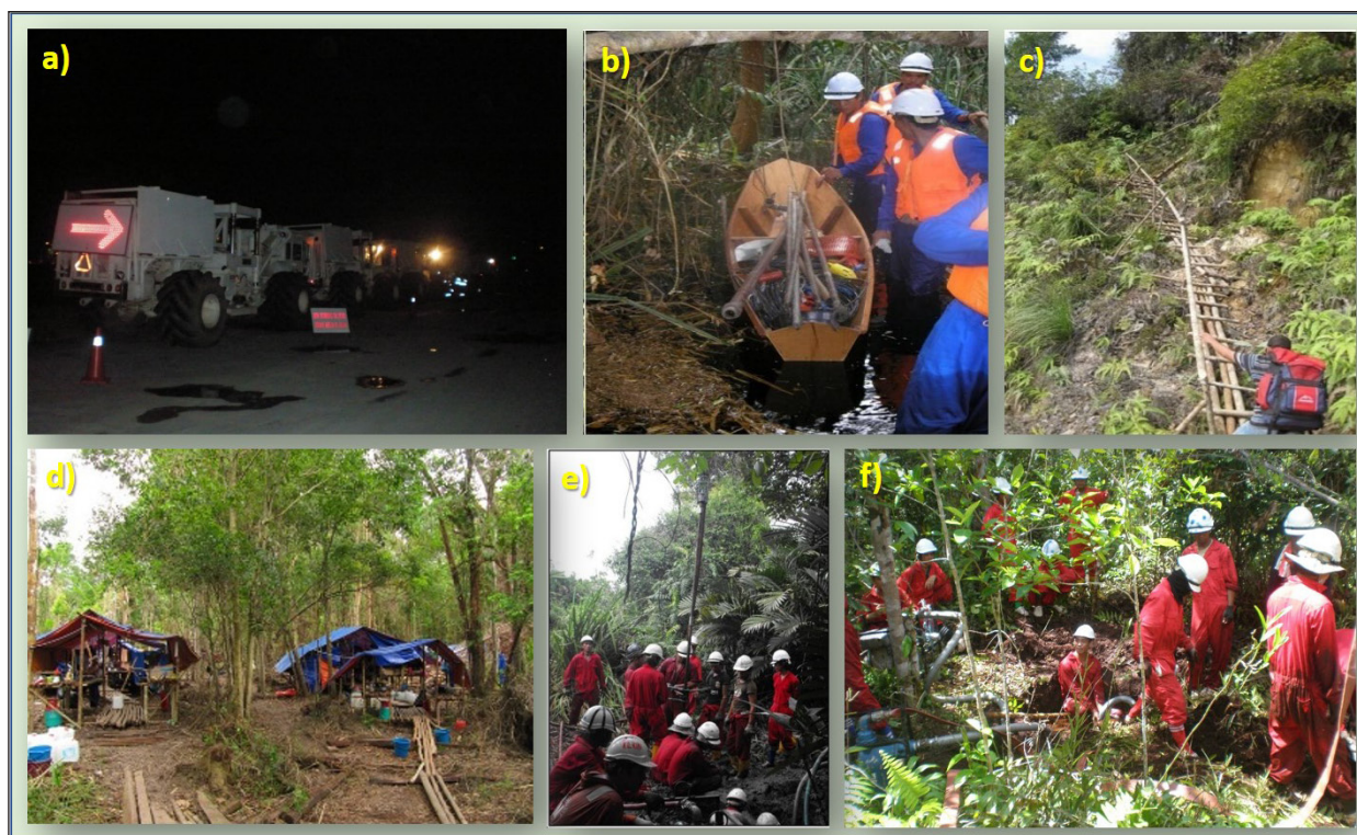
Figure 10: Seismic acquisition and operational challenges. a) Vibroseis operations at night, b) Laying geophones/hydrophones in swampy area, c) Bridging work with steep terrain in the hilly area, d) Fly camps for temporary living quarters, e) Up-hole drilling, and f) Shot-hole drilling.
