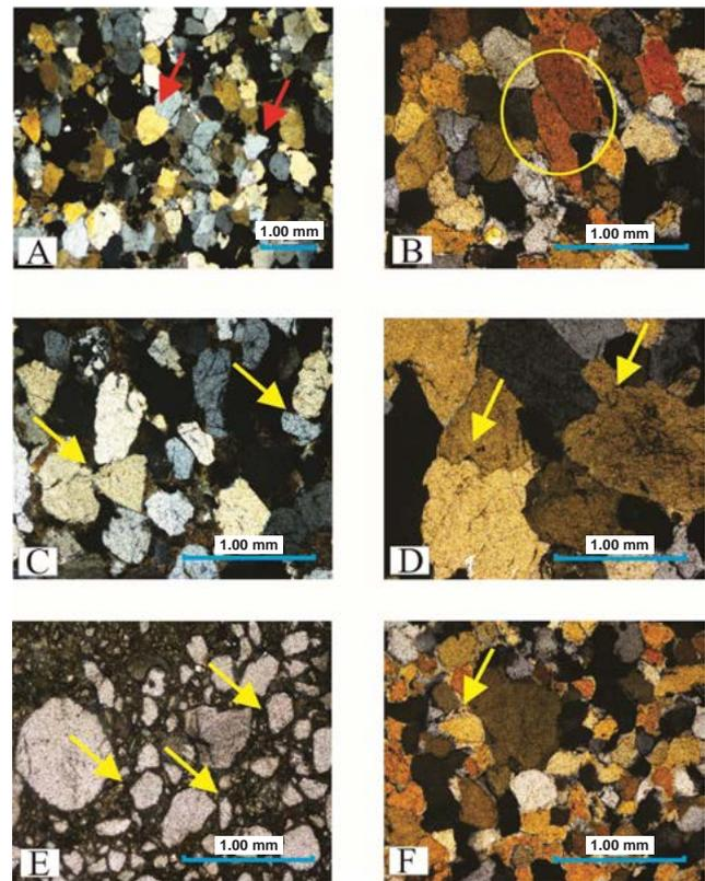
**Figure 4:** Diagenetic aspects from the Pab formation: (A) Convex-convex contact; (B) Plane contact; (C) Point contact (XP); (D) Intense compaction resulting in quartz suture contact; (E) Argillaceous pseudomatrix (XP); (F) Quartz overgrowth structure.
