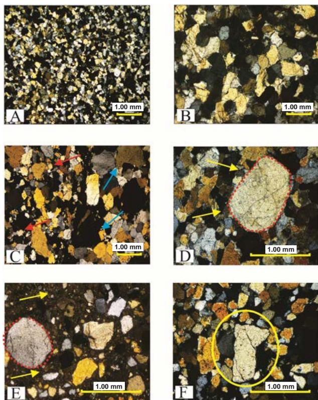
**Figure 2:** Textural variation and structure of the studied samples. (A) Very fine-grained, wellsorted, massive sandstone (crossed polarizers, XP); (B) Fine to medium sandstone (XP); (C) Medium grained, very poorly-sorted, massive sandstone (XP); (D) Coarse subrounded quartz grain with quartz overgrowth structure at the edges; (E) Mud Argillaceous intraclasts; (F) Fractured coarse grain angular quartz.
