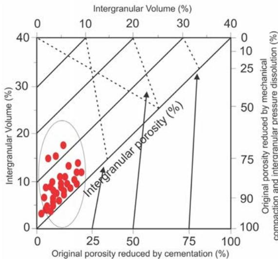
**Figure 6:** Ehrenberg (1989) diagram showing the relationship between intergranular volume and total cement, correlating the primary porosity reduction with cementation and/or compaction.
