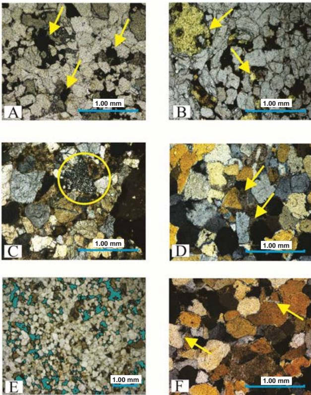
**Figure 5:** (A) Primary porosity widely preserved; (B) Argillaceous pseudomatrix and excavation pores; (C) Chert fragment; (D) Porosity reduction due to quartz overgrowth and dissolution of less competent clay minerals; (E) Preserved porosity (uncrossed polarizer); (F) Calcite cements resulting in porosity reduction.
