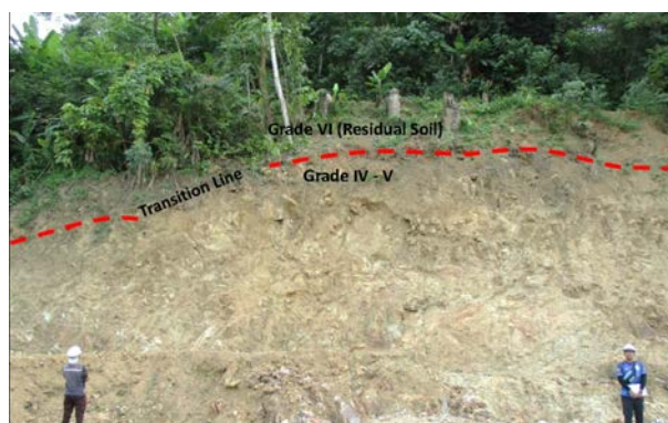
Figure 8: Overview of weathering profile of grade IV – V at circle C area of Figure 2.
